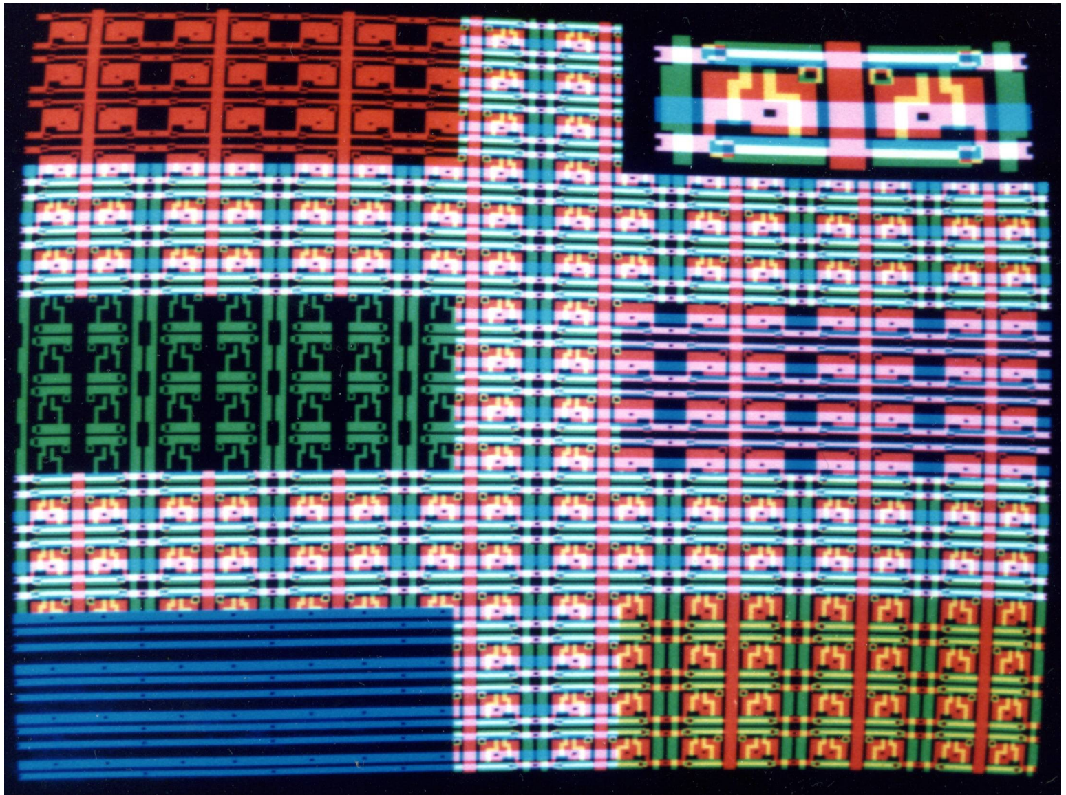
Photo mask layout design example of six transistor SRAM using N channel silicon gate E/D (Enhancement-mode for gate, Depletion-mode for load) MOS transistors for front cover of this issue
