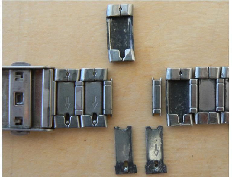
Removing Metal Section Block
