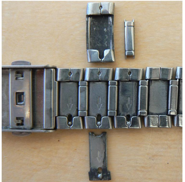
Removing Metal Section Block
