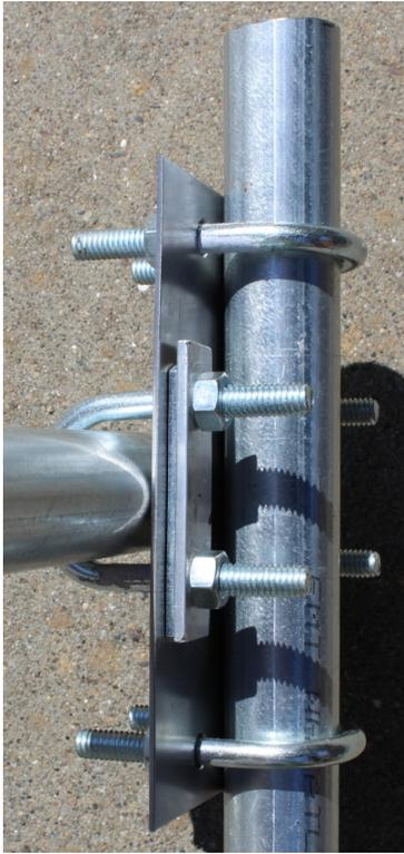
Antenna Mast Crossing by U-bolts and Steel Board
