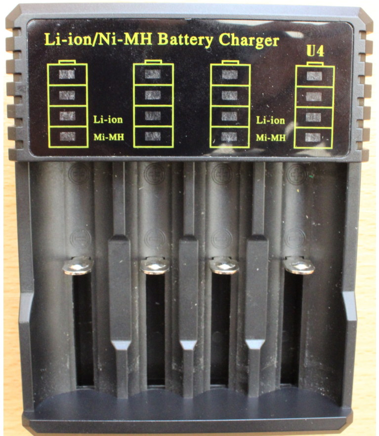
USB charger with four charge levels display
