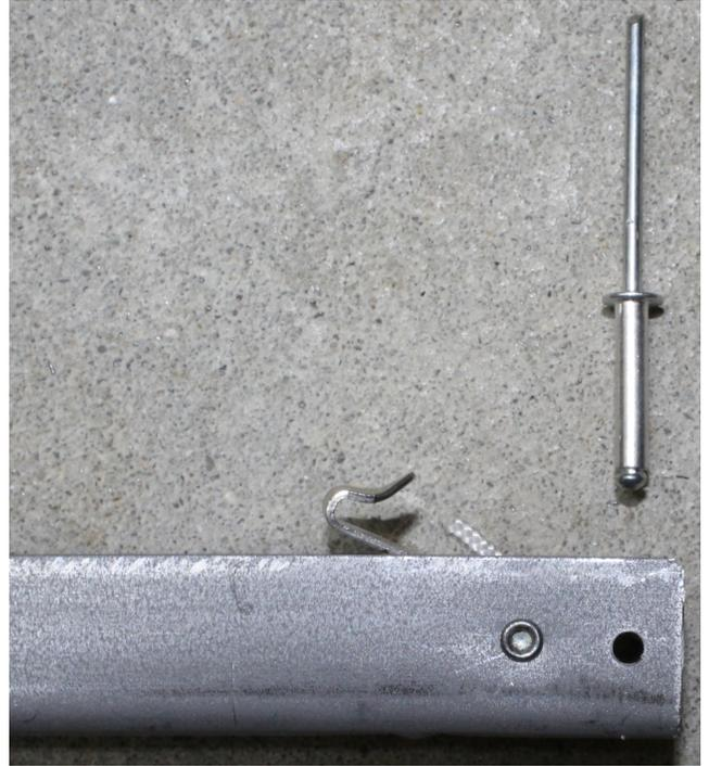
Rivet for Bottom Guide of New Channel Balance
