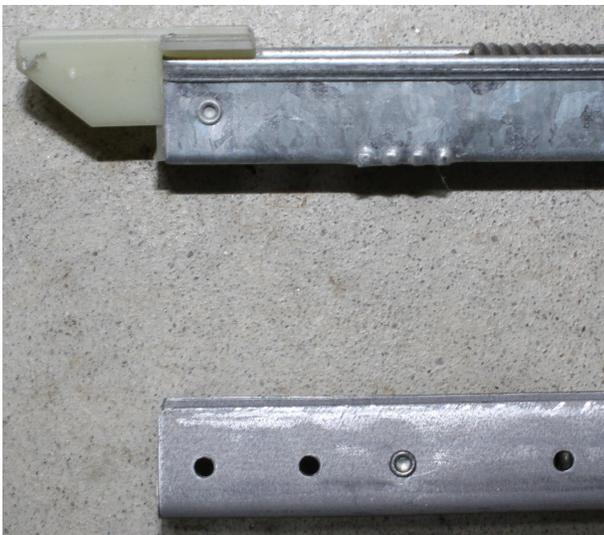
Top Guide on Broken Channel Balance to be Removed
