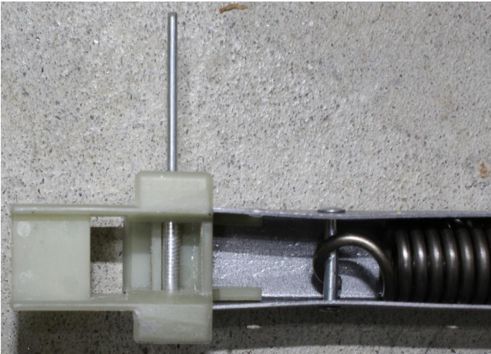
1/8" x 5/8" Rivet Passed through Hole to be Fixed
