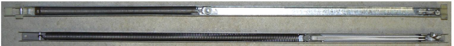
Broken Channel Balance with Guides (Upper), New Channel Balance without Guides (Lower)
