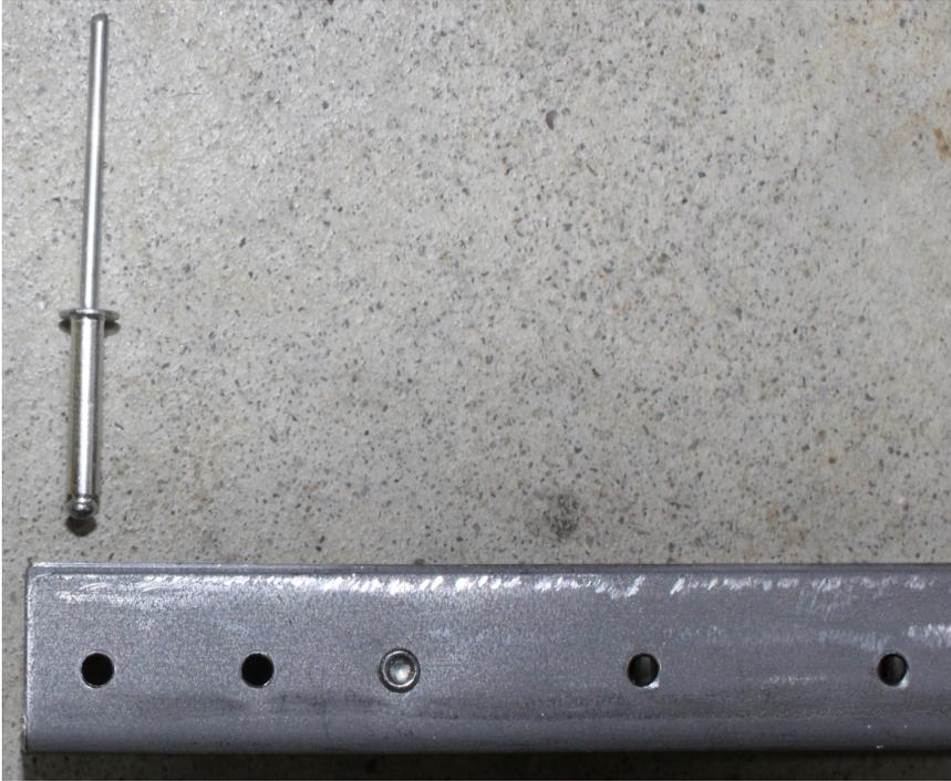
1/8" x 5/8" Rivet for Top Guide of New Channel Balance
