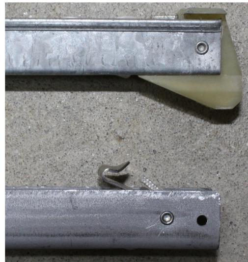
Bottom Guide on Broken Channel Balance to be Removed
