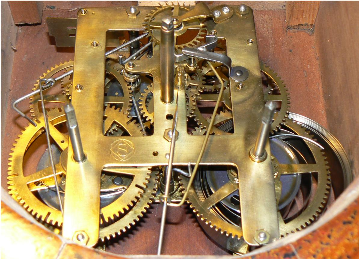
Clock Mechanism (Pawl Rod for Main Spiral Torsion Spring (Right) Broken, Pawl for Chime Spring (Left) Intact)
