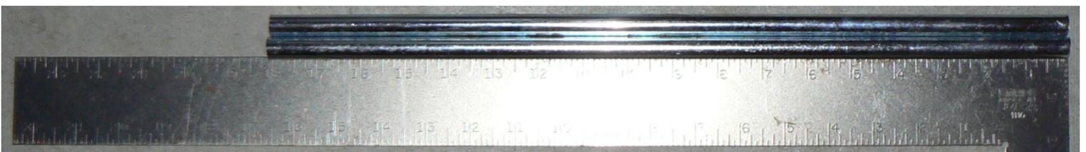
Torsion Spring Winding Tool (Two 18" Steel Rods)
