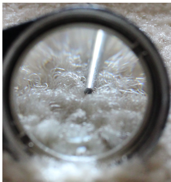
Opening of capillary tube
