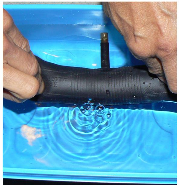
Air Bubbles from Tube Punctured
