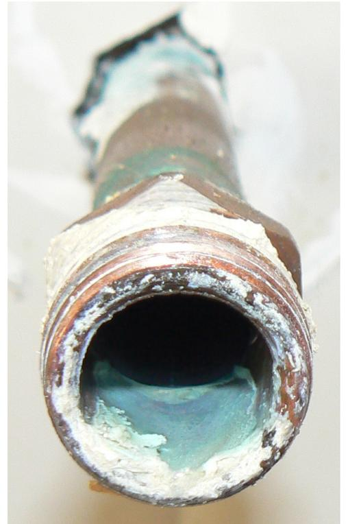
Sediments in 1/2" Copper Pipe Inlet
