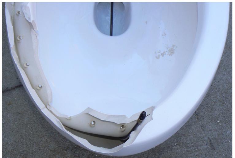
Flush Water Flows Rear Surface of Bowl and Drain
