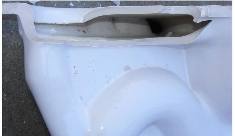
Flush Water Inlet (Cross Section View)
