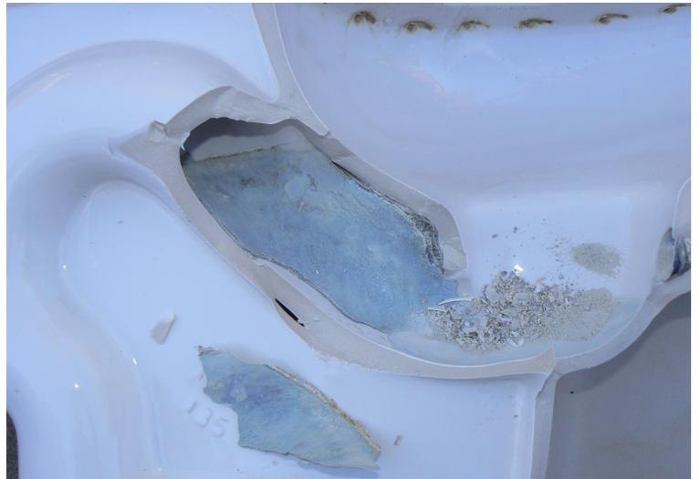
Drain Path until Water Level Filled with Scale Deposited
