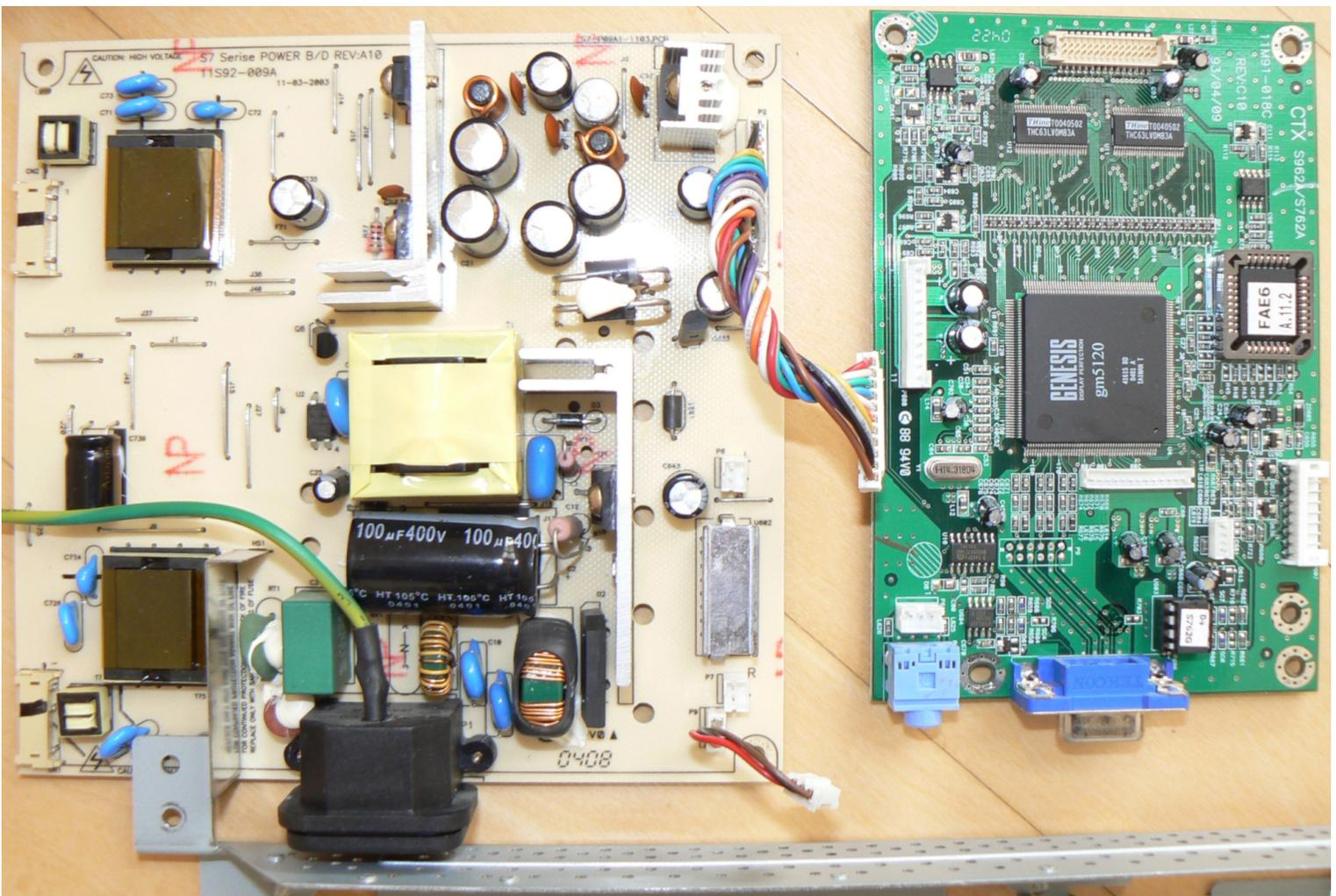
Power Supply & Controller with VGA video connector & Audio Connector
