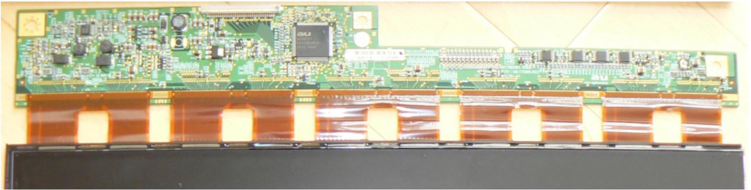
Row & Column Drivers and LCD Flat Panel Connected by FFC (Flexible Flat Cable)
