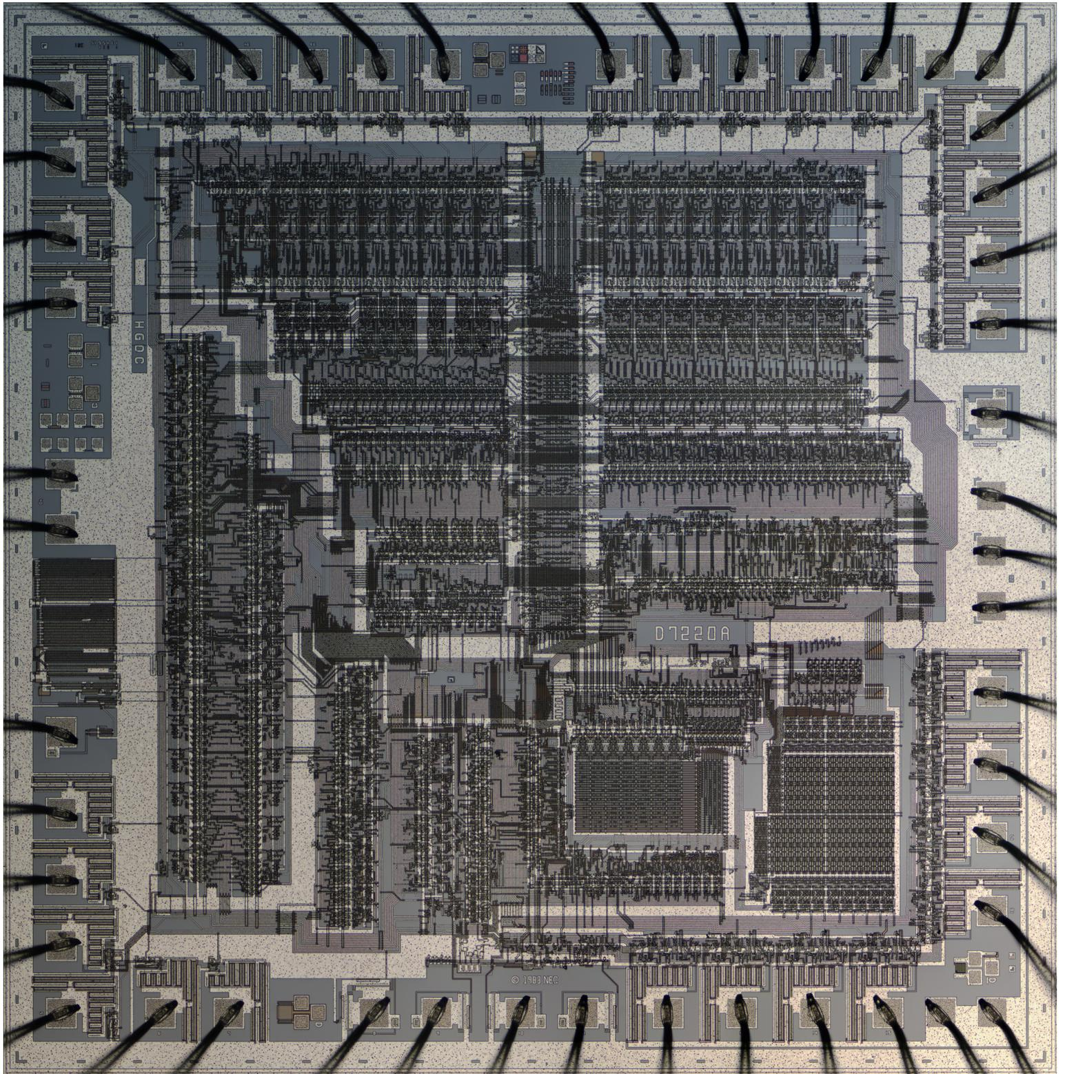
μPD7220A 20x Die Photo 15709 x 16000 (251MP) 6400% (64x) Tolerant Synthesized by Hugin
