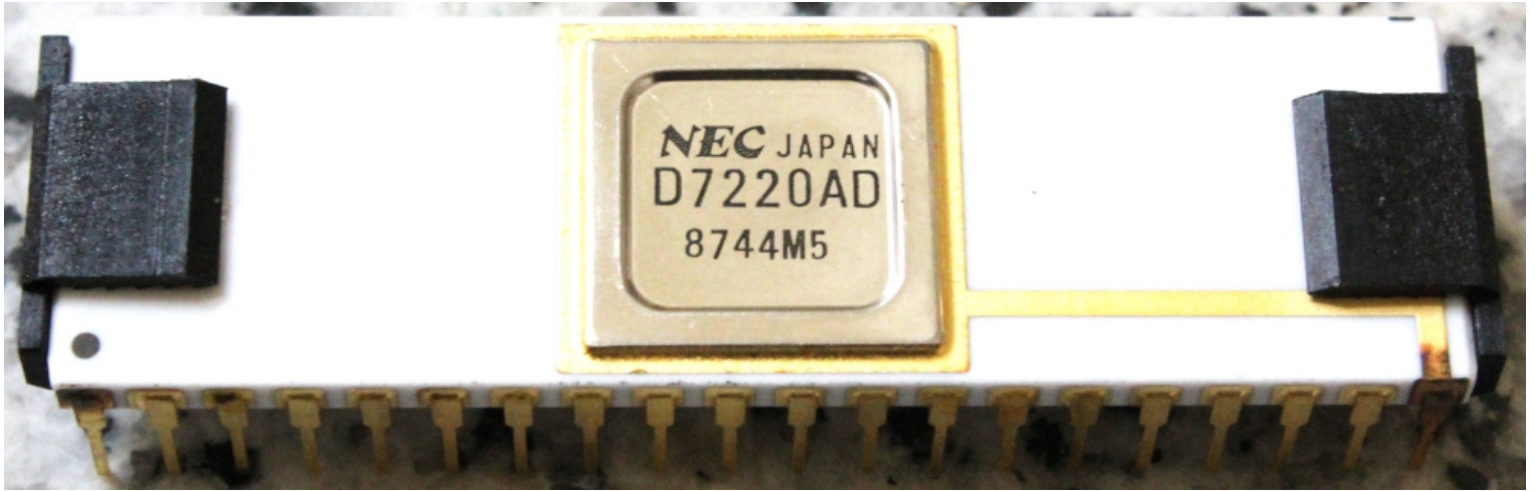
\mu PD7220A (manufactured in 1987 44 th week) Encapsulated in Ceramic DIP Package before Decapsulation ( \mu PD7220A was still under mass production even after I designed and resigned from NEC in August, 1987)
