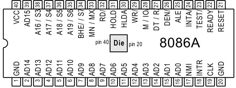
Pin association of next page die photo exactly reflects the die position mounted on the island of the base ribbon.
