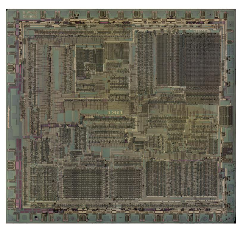
80C86A 20x Die Photo 14000 x 13055 (183 MP) 6400% (64x) Tolerant Synthesized by Hugin
