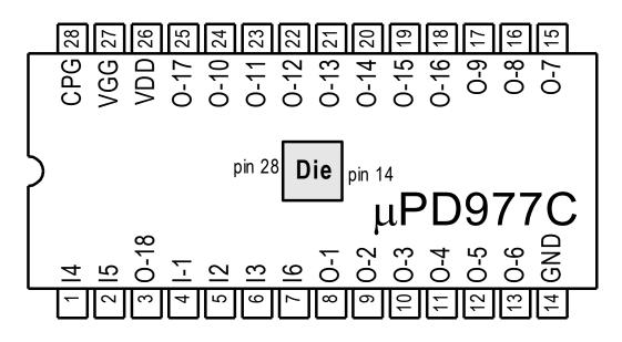
Pin association of next page die photo exactly reflects the die position mounted on the island of the base ribbon.
