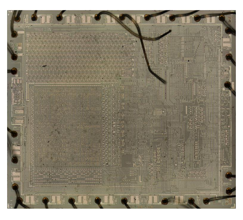
$\mu PD946C$  20x Die Photo 17500 x 15165 (265 MP)  $\,$  6400% (64x) Tolerant Synthesized by Hugin
