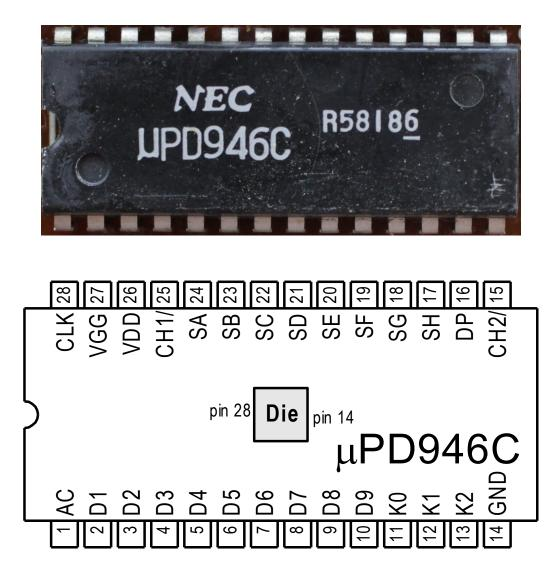
Pin association of next page die photo exactly reflects the die position mounted on the island of the base ribbon.
