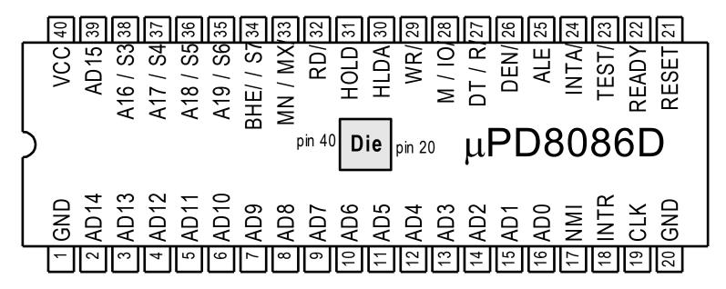
Pin association of next page die photo exactly reflects the die position mounted on the island of the base ribbon.
