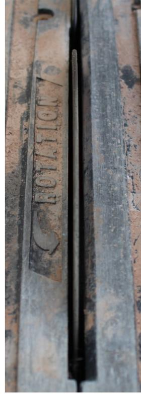
Saw Blade is Cooled by Water Rotating through Water Tank Stored under the Deck Plate
