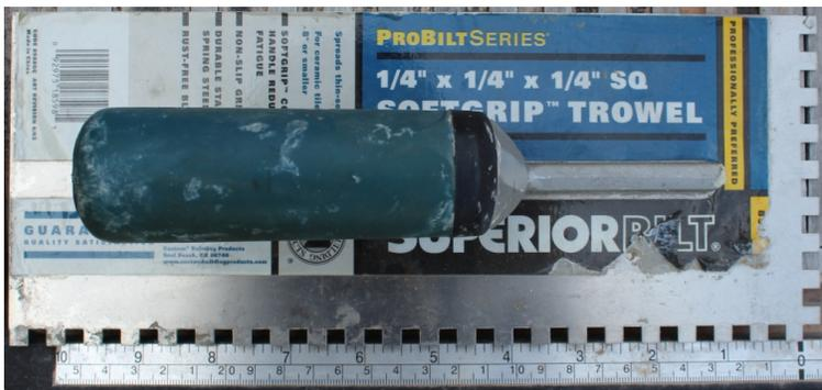
Trowel with 1/4" x 1/4" Openings for Aligning the Adhesive Height between Tile and Floor
