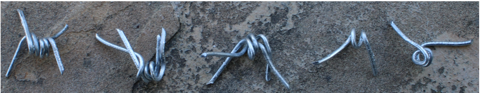
Four barb pairs removed (A barb consists of two short pins with 2 edges 30 degrees sliced reversely)
