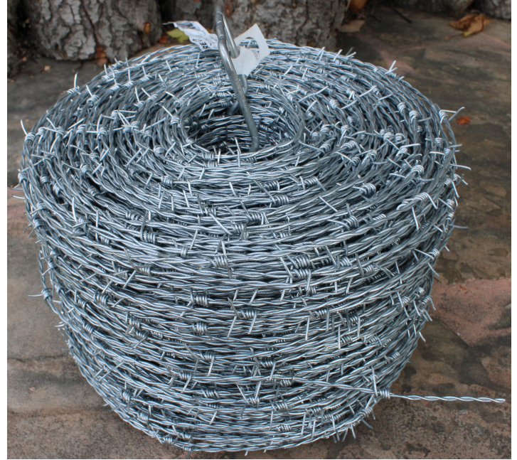
A roll of barbed wire (15.5 Gauge, 4 points Barb 5" Spacing, 80 Rods (1,320'), 42lb, Zinc coating class 3)
