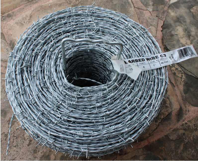
A roll of barbed wire (15.5 Gauge, 4 points Barb 5" Spacing, 80 Rods (1,320'), 42lb, Zinc coating class 3)
