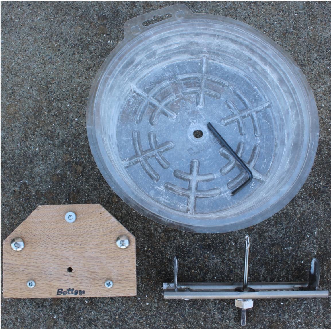
Two Boards with 5 Bolts & Nuts (Handmade), Hole Cutter & Plastic Tray (Commercially Manufactured)
