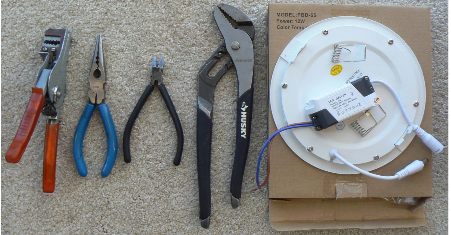
Wire Stripper, Long Nose Plier, Diagonal Cutter, Groove Joint Plier, 6" LED Light Module with Rectifier
