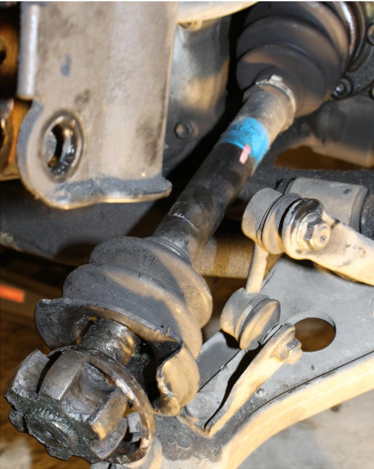
Broken CV Joint & Replaced Stabilizer Link Set Bracket
