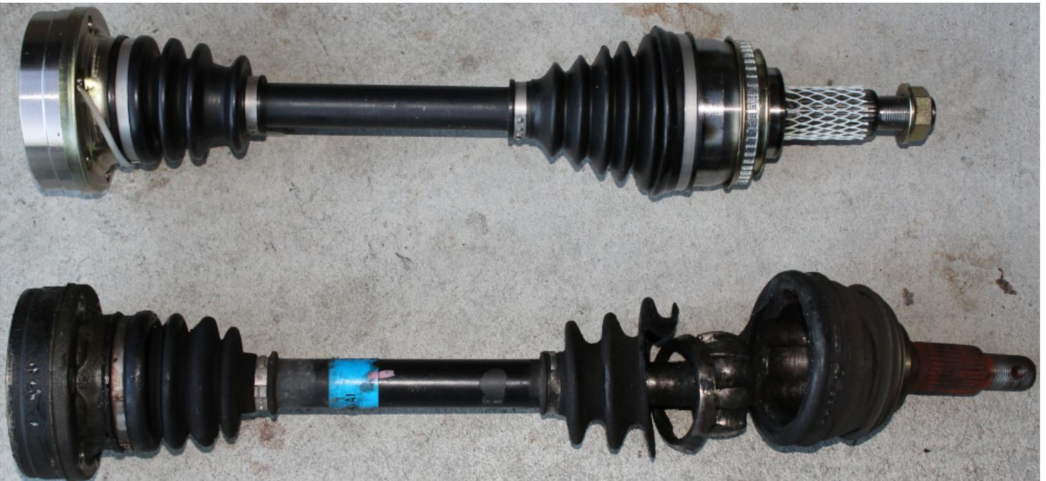
New Drive Axle with CV Joint (Top) & Old Drive Axle with Broken CV Joint (Bottom)
