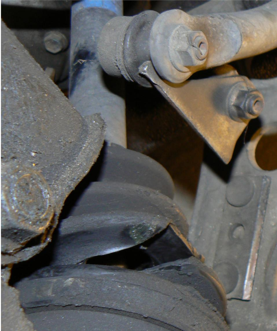
Broken Stabilizer Link Set Bracket (Right) & Broken CV Joint Sleeve (Bottom)
