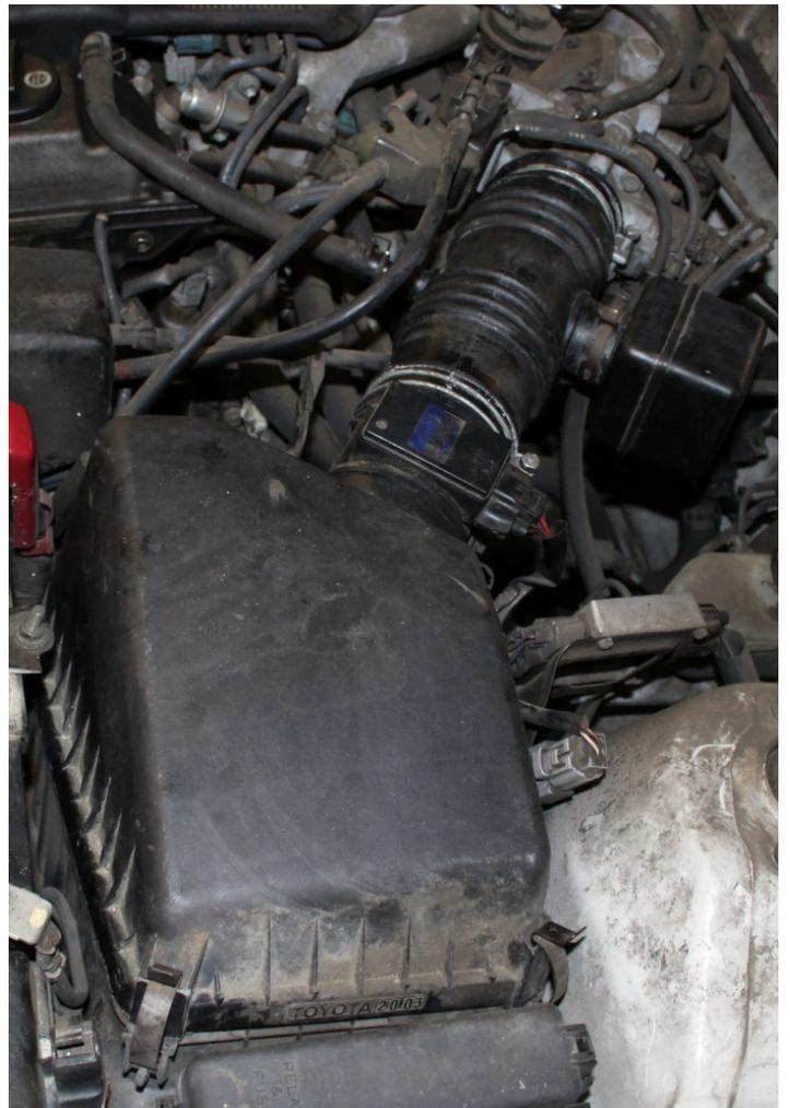
Replaced Air Filter (Bottom) & Tube (Center Right)
