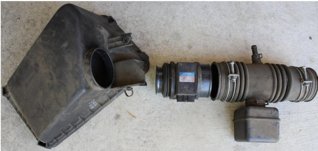
Mass air flow sensor itself is working well (No need to replace).
