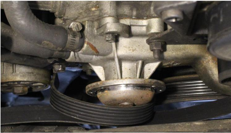
Drive Belt Released & Pulley Removed
