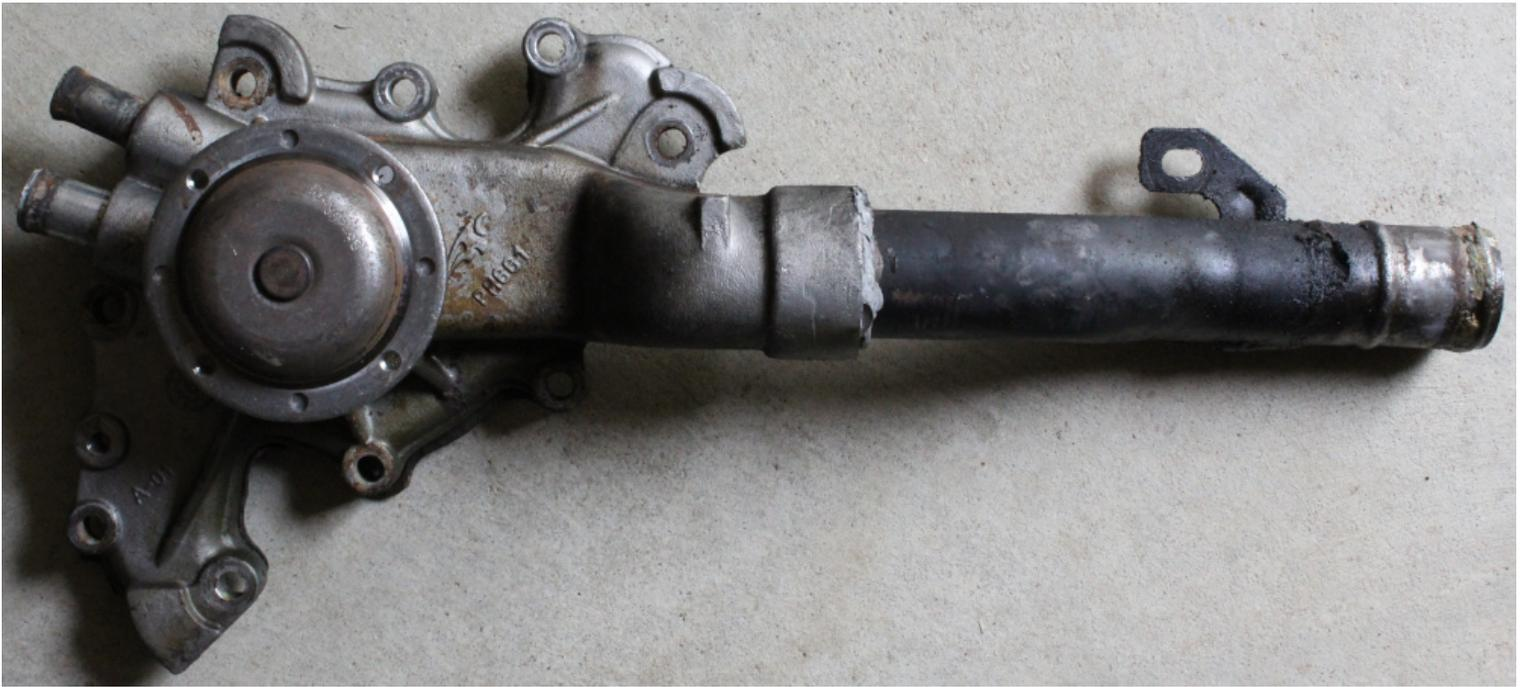
Old Water Pump with Inlet Tube Removed
