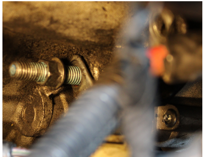
Removing Stud Bolt#1 along with ground wire
