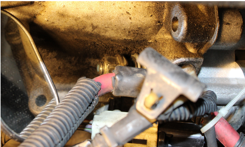
Bolt#2 (left) & Stud Bolt#1 (center), Stay-hole (up-right)
