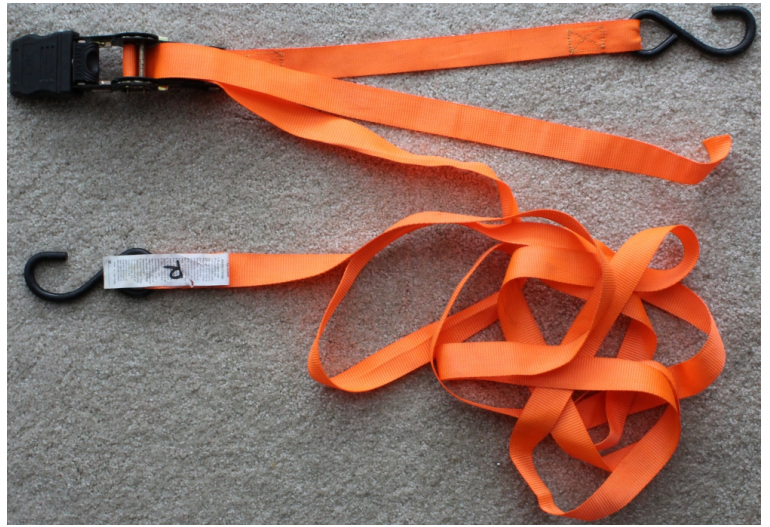
Seq. 4 (Open ratchet; Pull strap to adjust strap length)
