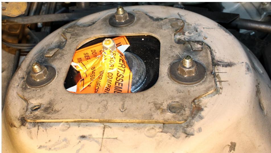
Fastened new strut assembly by three strut mounting nuts on shock tower
