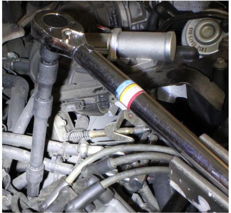
Releasing Engine Mount Nut from Engine Room
