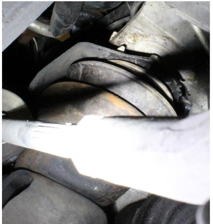
Top of the Engine Mount Released from Engine Chassis
