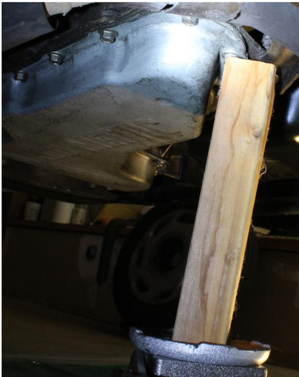
Pushing up the Engine through Oil Pan
