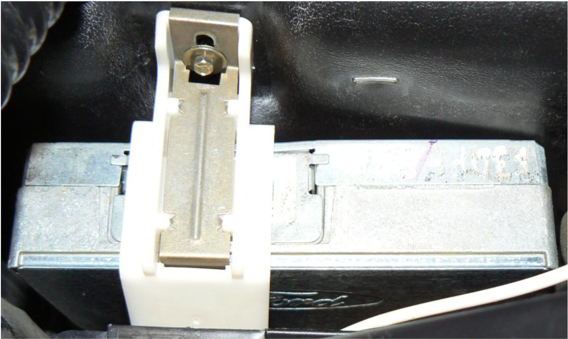
Engine Control Module Support
