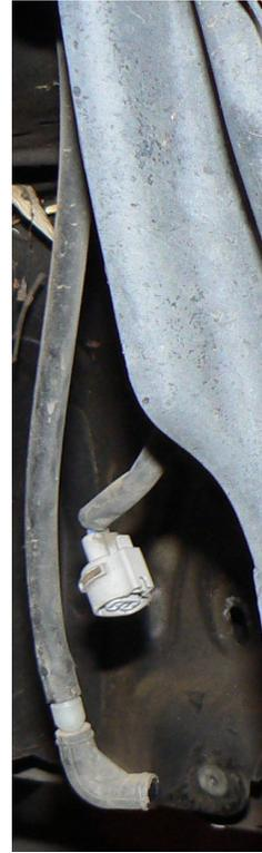
Fluid Outlet Connection & Pump Connector Removed
