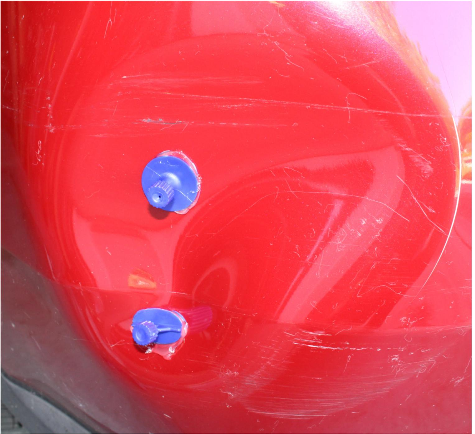
Dent Repair Trial by Pulling the Dent (Failed)
