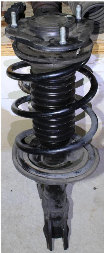
Assembled with New Boot, Dump Stop & Spring
