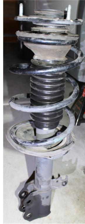
Assembled with New Boot, Dump Stop & Spring
