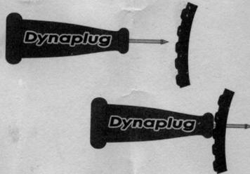
6. Pull tool from hole. Plug will remain in hole. For most punctures from nails and screws, one plug is sufficient.
