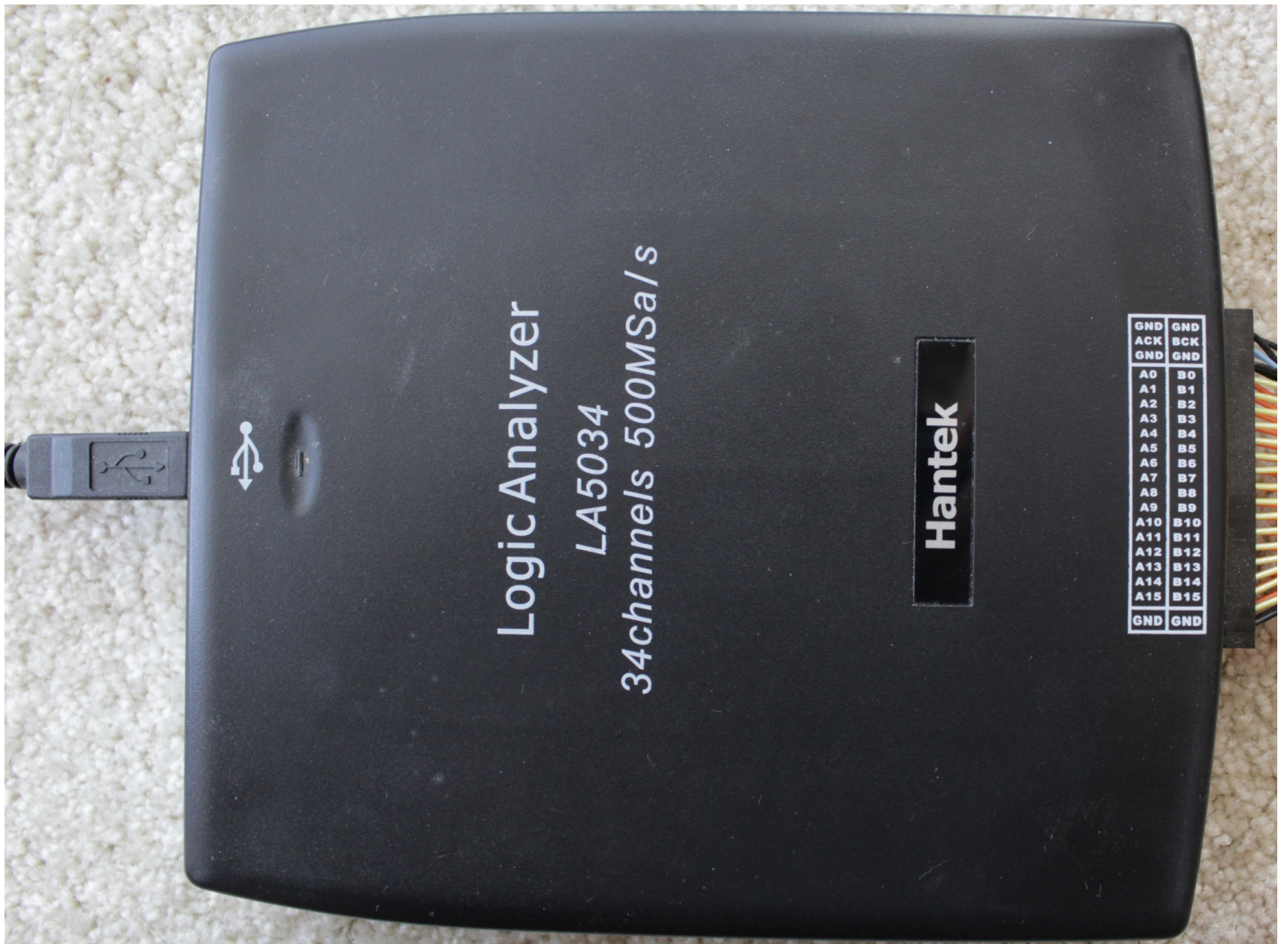
Hantek Logic Analyzer (34 channels, 500M Samples per Second)
