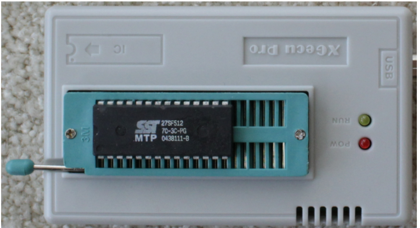
Xgecu TL866II Plus Programmer with 40 Pin Dual Inline Zero Insertion Force Socket
