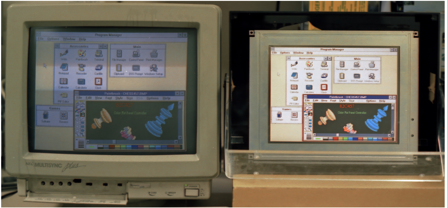
Simultaneous display on 14" CRT monitor TV (NEC MultiSync Plus) & 10.4" Sharp TFT (Thin Film Transistor) color flat panel (Display quality of digital flat panel was much better than analog CRT (Cathode Ray Tube)) Demonstrating the transition from CRT to Flat panel
